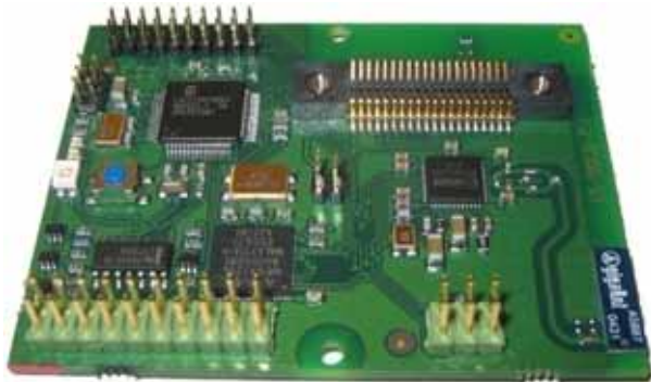
Connect Blue Sensor Routing Node ARM7 – 32K RAM, 512K flash
